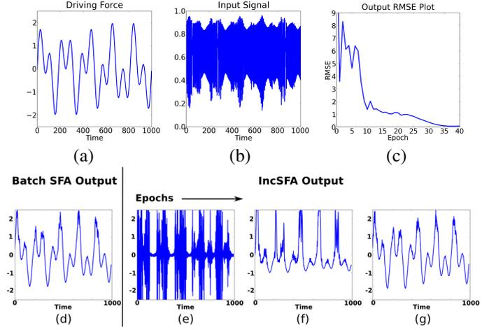
Figure 2: Experiment conducted on a chaotic time series derived from a logistic map. A learning rate of  $\eta = 0.004$  was used. (a) Driving Force (b) Input (c) Output RMSE plot (d) Batch SFA output of the slowest feature (e)-(g) IncSFA output at  $t = 15, 30, 60$  epochs.
