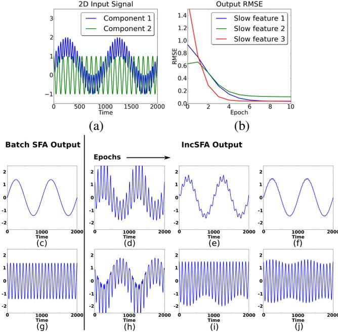
Figure 1: Experiment conducted on a simple non-linear input signal. A learning rate of  $\eta = 0.08$  was used. (a) Input Signal (b) Output RMSE plot (c) Batch SFA output of the first slow feature (d)-(f) IncSFA output at  $t = 2, 5, 10$  epochs. (g) Batch SFA output of the second slow feature (h)-(j) IncSFA output at  $t = 2, 5, 10$  epochs.
